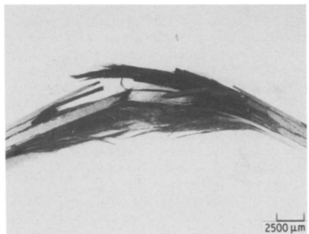
Figure 13 Optical photograph of 0° SiC-reinforced LAS-II tested in air at 900°C after 66 h at 364 MPa (residual strength = 620 MPa).
